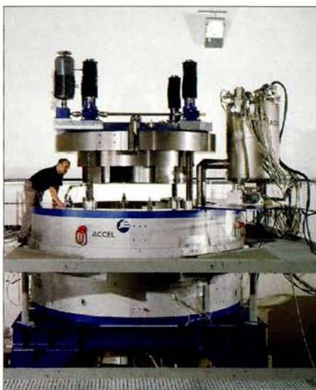
The superconducting proton cyclotron (left) developed by ACCEL, and its associated gantry.
