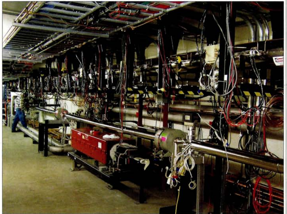
The Recycler storage ring (inside black brackets) and its electron-cooling system are located just above Fermilab's Main Injector accelerator (bottom, with red quadrupole magnet). The shiny pipe in the middle is the electron-beam return line. (Courtesy Fermilab.)
